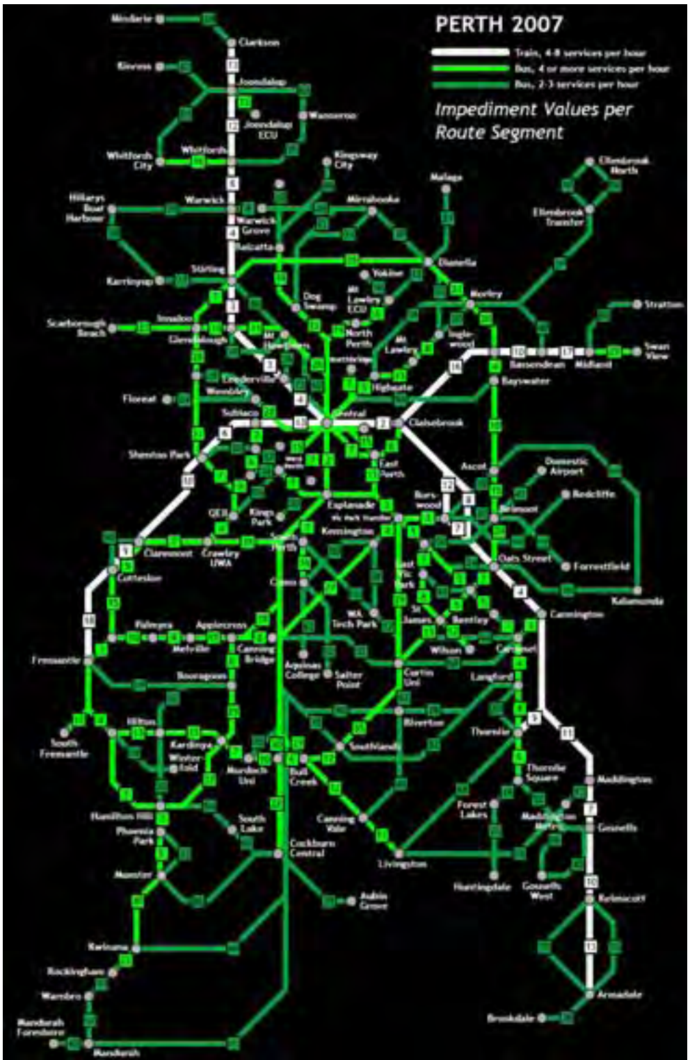
Map 14: Public transport in Perth before opening of the Perth to Mandurah railway, with modes, service levels and impediment values per route segment.
